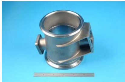
Sintered Boeing Airliner Component
